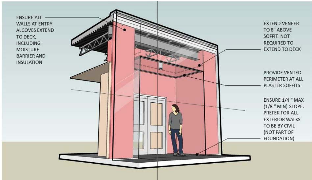
Diagram 07_01 (Refer to Division 07) – Completion of Moisture and Thermal Envelopes at Exterior Alcoves
